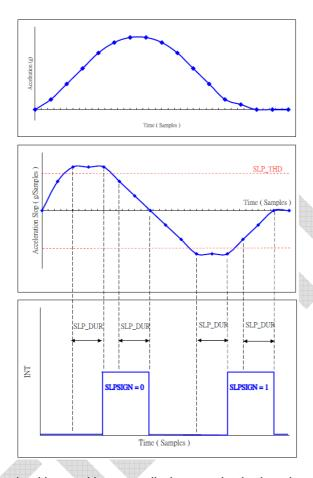
Note1: In order to ensure motion algorithm working normally, interrupt latched mode must be set before motion algorithms enabled.
