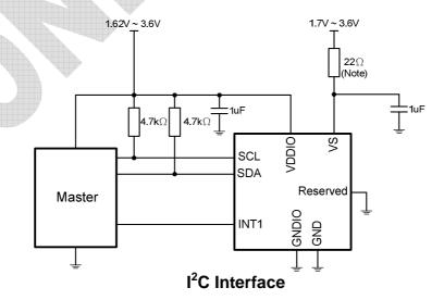
Note: A 22 ohm resistor is recommended to filter out the system power noise.
